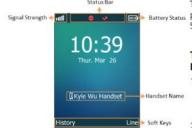
The LCD screen is divided into three parts: Status Line, Text Line and Softkey Line.
